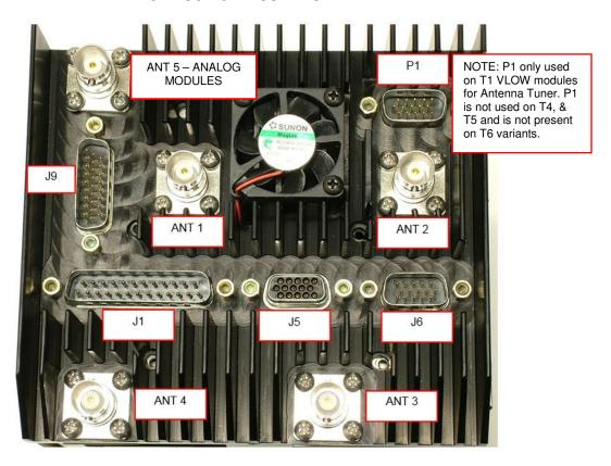
FIGURE 2: TDFM-9300 Antenna & Connector Locations
