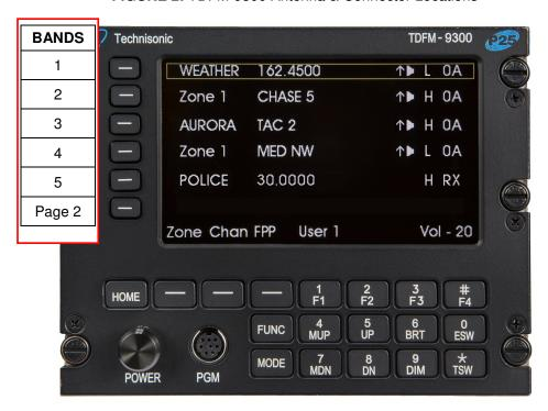
FIGURE 3: TDFM-9300 Band Display Orientation
