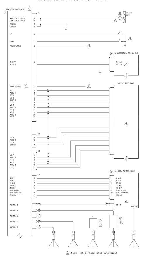
FIGURE 4: Wiring Connections for Individual Band Control
