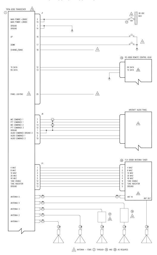
FIGURE 5: Wiring Connections for Combined Band Control
