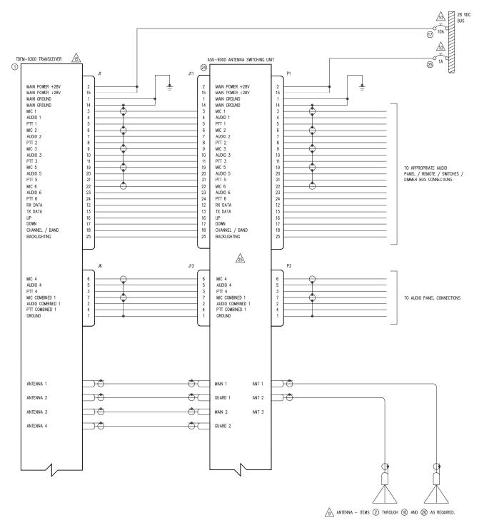
FIGURE 7: Wiring Connections for ASU-9000
