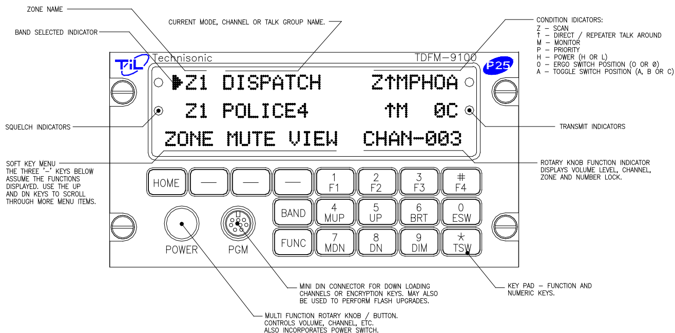
FIGURE 1: Front Panel Controls – TDFM-9100 Transceiver
