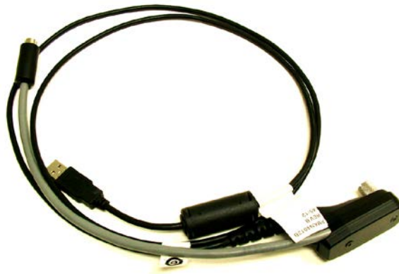
FIGURE 3: Programming Cable: “PC-9000” P/N 127499
